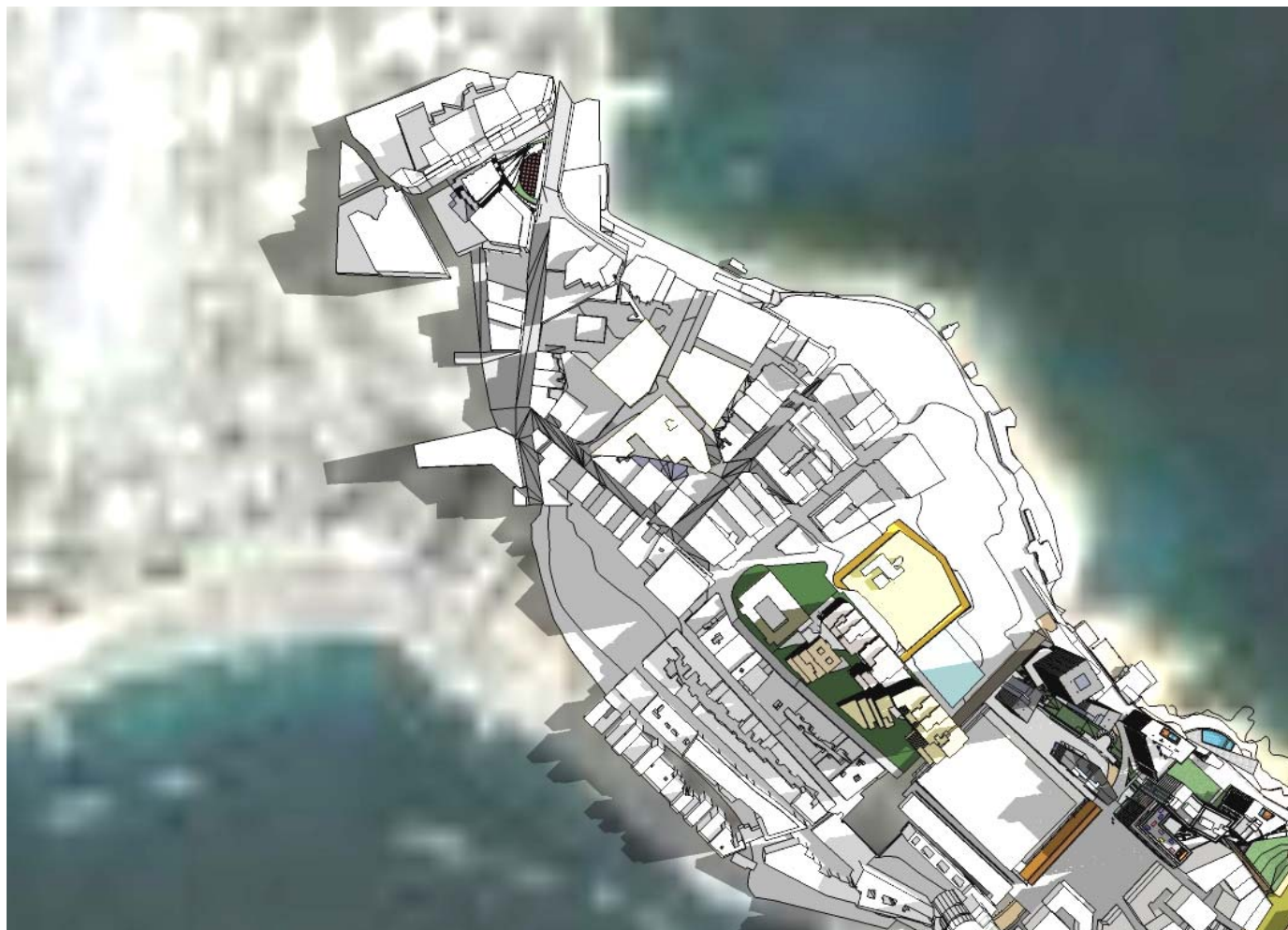
Figure 29: Shadowing: 21 July: Traditional Housing (1 hour after sunrise)
