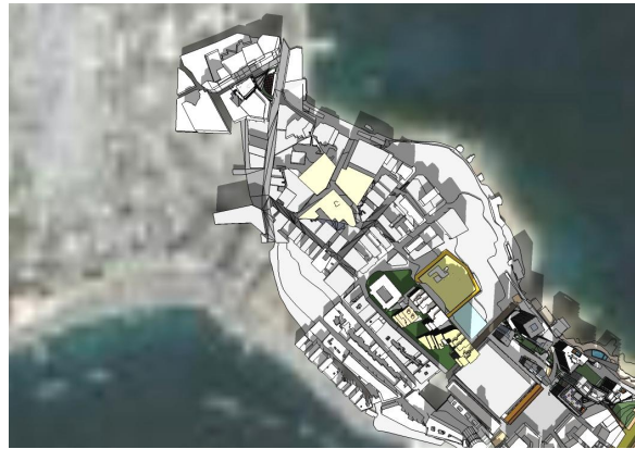
Figure 2.3: Shadowing: 21 November: Traditional Housing
