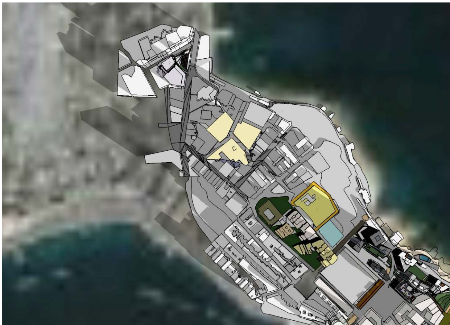
Figure 1: Shadowing: 21 November: Traditional Housing (1 hour after sunrise)
