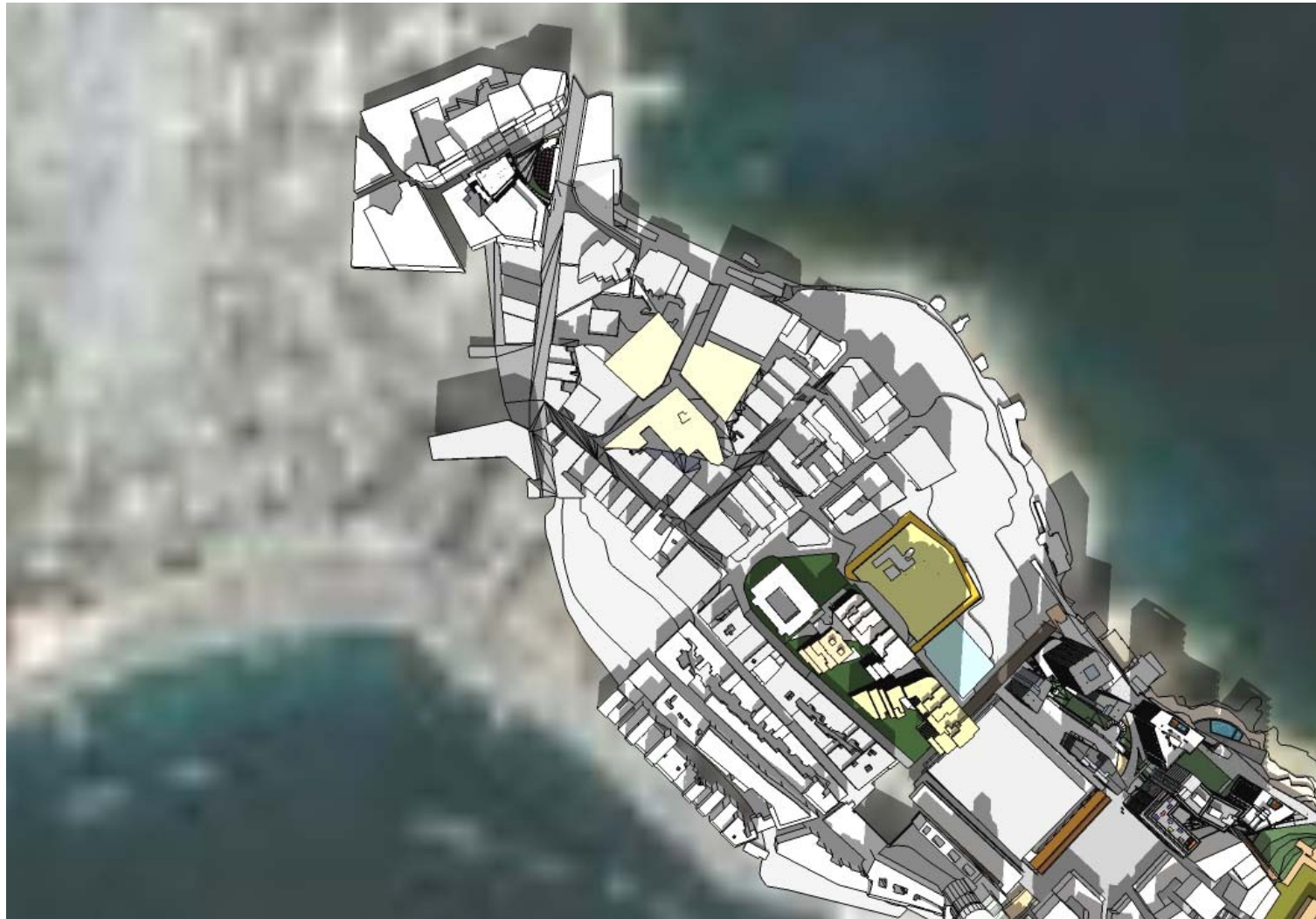
Figure 2: Shadowing: 21 November: Traditional Housing (noon)
