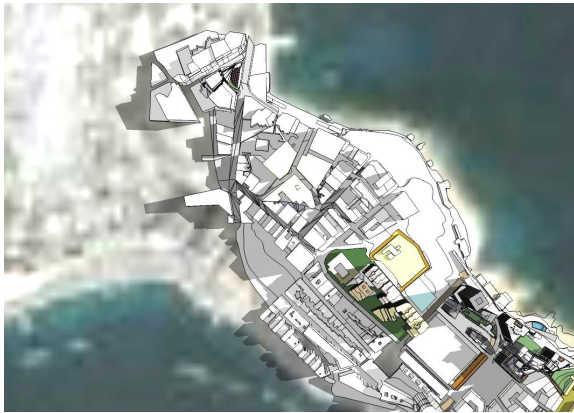
Figure 2.14: Shadowing: 21 July: Traditional Housing
