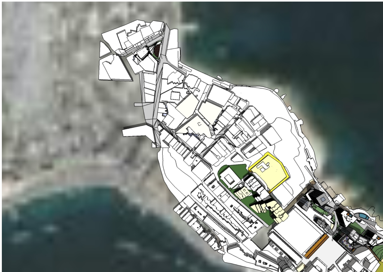
Figure 29: Shadowing: 21 July: Traditional Housing (noon)
