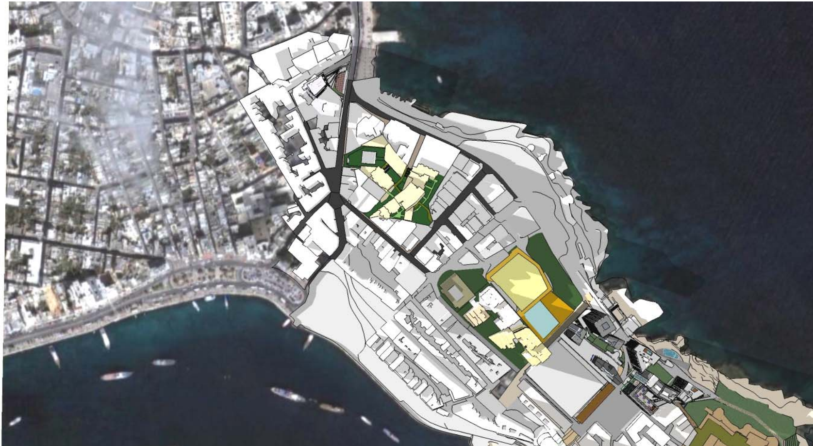
Figure 33: Shadowing: 21 July: Scheme (1 hour before sunset)
