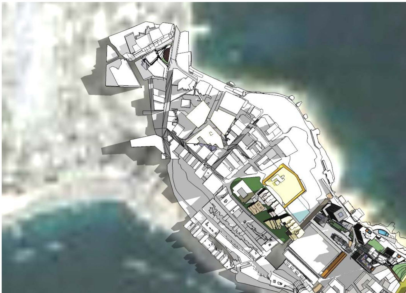
Figure 25: Shadowing: 21 June: Traditional Housing (1 hour after sunrise)
