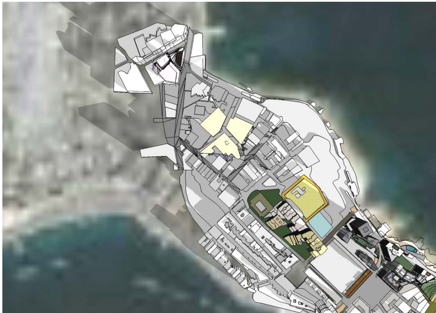
Figure 13: Shadowing: 21 January: Traditional Housing (1 hour after sunrise)
