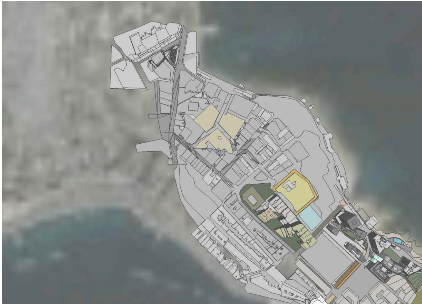
Figure 25: Shadowing: 21 June: Traditional Housing (1 hour before sunset)
